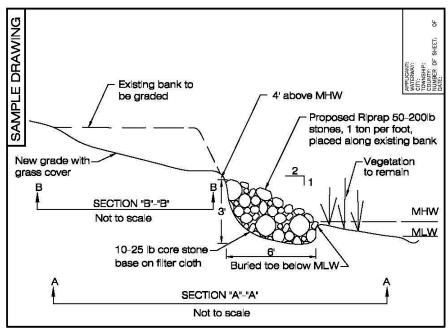
Riprap Revetment & Associated Backfill
